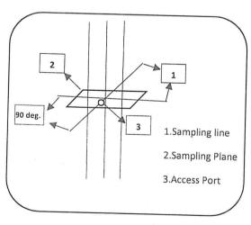
2. Number of sampling ports: Minimum two (at 90 degrees) sampling ports are required in a circular chimney, so that full stack cross-sectional area can be covered for measurements. For stacks having diameter between 2 and 4 meters, two mutually orthogonal sampling ports are to be increased to four by providing additional sampling ports at diametrically opposite position, to the first two sampling ports.
